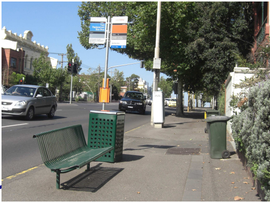
Public transport waiting area No shelter is provided. Lack of tactile pavement, which leads to confusion where passengers are to be picked up and dropped off
