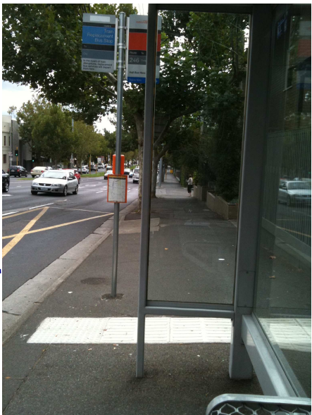
Public transport waiting area Edge of shelter located close to edge of traffic lane. Pedestrians walking through at this point may feel uncomfortable, due to proximity of fast moving traffic
