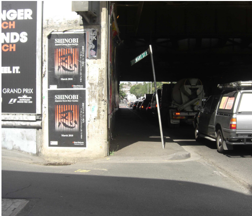
Stewart Street / Punt Road intersection Pedestrians are vulnerable at this crossing as vehicles turn into Stewart Street at speed. No tactile pavement is provided.
