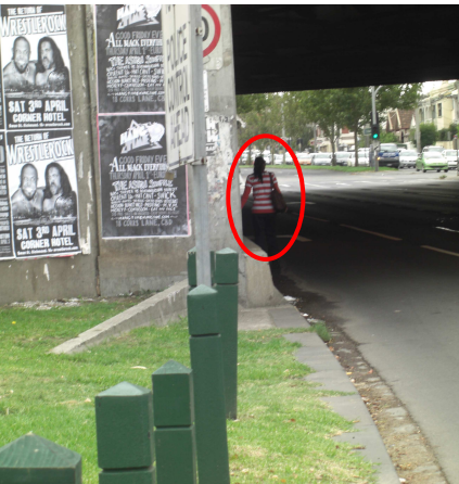
Tunnel – western side Pedestrians observed to walk in tunnel along western side. No footpath provided for pedestrian desire line from Olympic Boulevard to Brunton Avenue.
