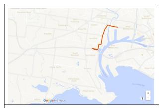
**West Gate Distributor (WGD)** – a 4km 4-lane road connecting the West Gate Freeway to Footscray Road, allowing trucks to bypass residential areas of the inner west. Sections of the WGD would be elevated (Hyde St, Francis St & Whitehall St). Estimated cost: up to \$0.5 Billion
